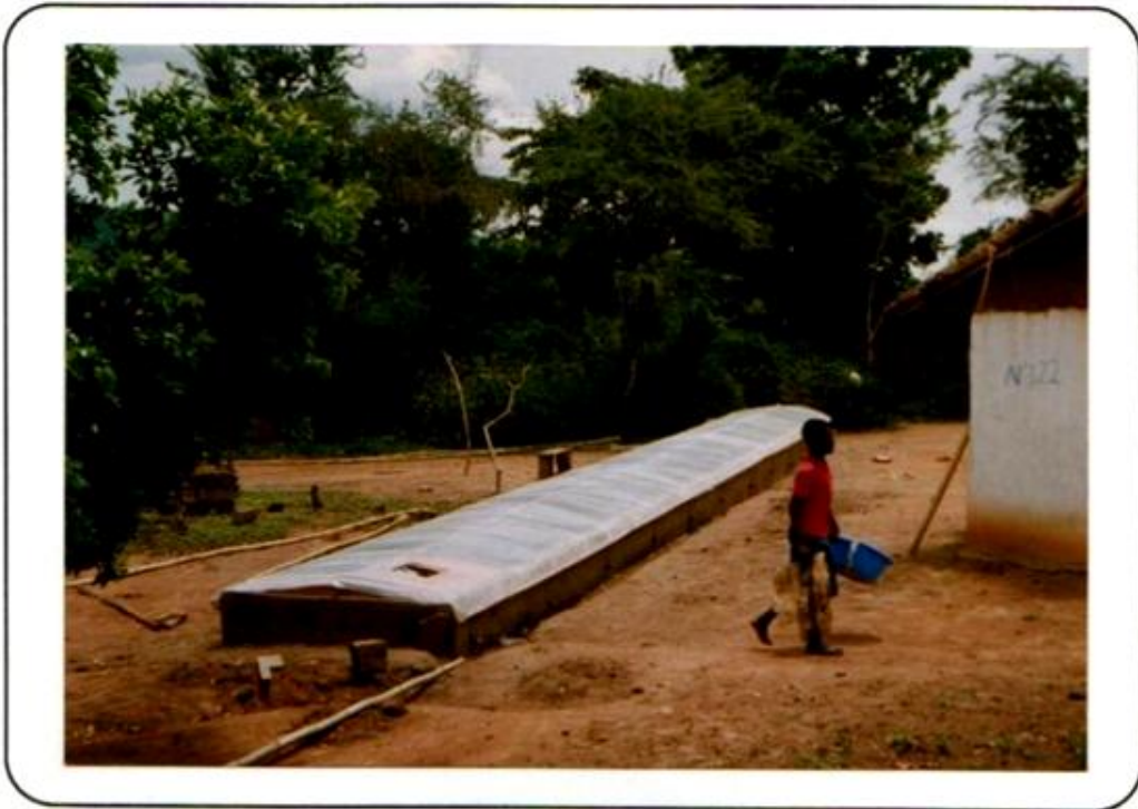
The finished dryer is aerated by a car ventilator. The latter gets its energy from a 50W solar module,
