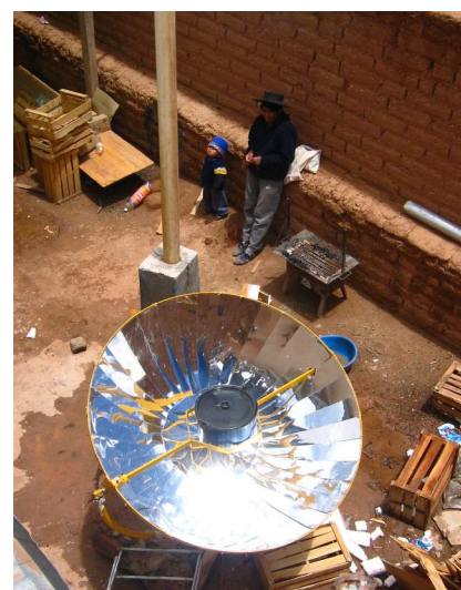
Fig. 9: Solar community cooker under construction in Cusi Cusi, and smaller parabolic cooker in the kindergarten.
