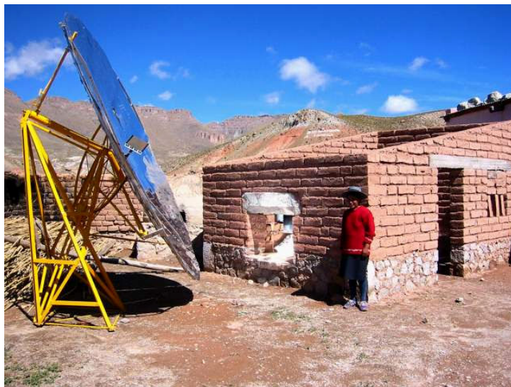
Fig. 8: Solar community cooker for the children's meals in Cienaga under construction, and using it to cook lunch for 40 children
